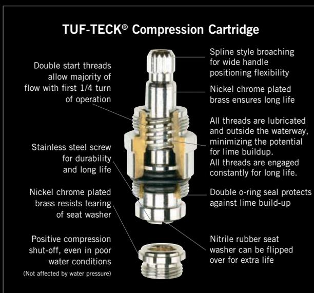
Double start threads allow majority of flow with first 1/4 turn of operation
