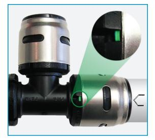
**STEP 3** Ensure that the pipe is pushed into the fitting fully and engaged properly by checking that the green indicator ring is fully visible in all four slots. This ensures a permanent connection.
