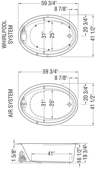
(  $\triangle$  ): Indicates suction positioning All dimensions are approximate. Structure measurements must be verified against the unit to ensure proper fit.
